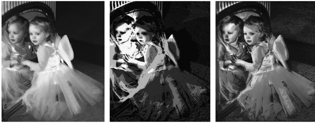
Fig. 6. Application of our method to a very diffusely lit image. In this example we aim to obtain different moods by changing the light environment and the degree of stylization. Left: Original input image. Middle: A very stylized and dark version of the input by multitoned depiction with four point light sources at (140,400,300), (140,400,350), (140,400,400) and (140,400,900) and using (F_b, F_d)=(1.0,0.2) . Right: Less stylized depiction obtained by combination of multitone and color relighting effects with lights at (134,530,290), (115,15,270), (315,695,350), (100,400,1000) and (589,325,325). No mask was used for these depictions.
